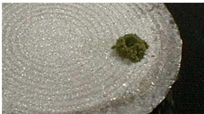
Instead of curly metallic shavings, a green powder came out of the hole! By looking in the drilled hole it was now clear that the metallic faces on the object were just thin coatings. The object was apparently composed of a dark greenish material throughout.
