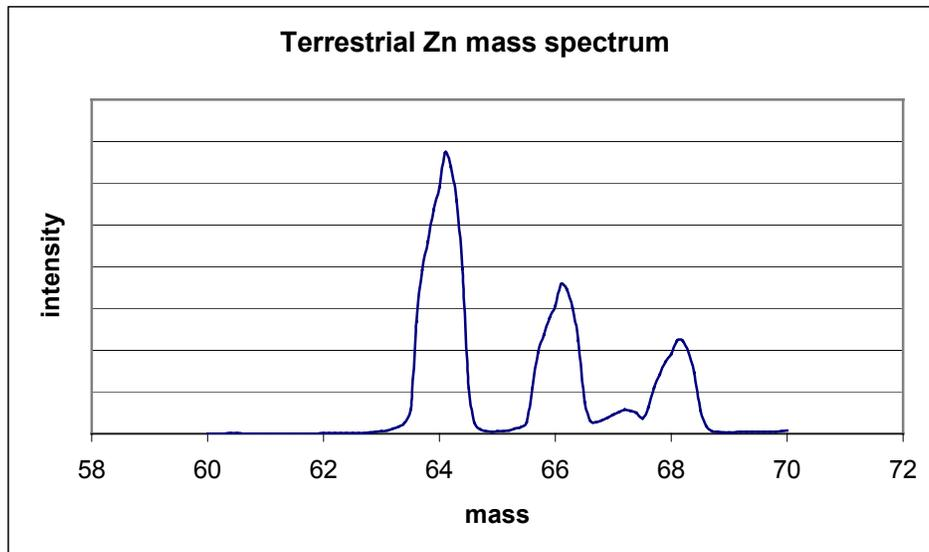
The observed peak intensities in this spectrum match the expected terrestrial abundance of these Zn isotopes reasonably well (within 15% relative). As a result, it was decided to remove a similar shaving sample from the object by drilling.
